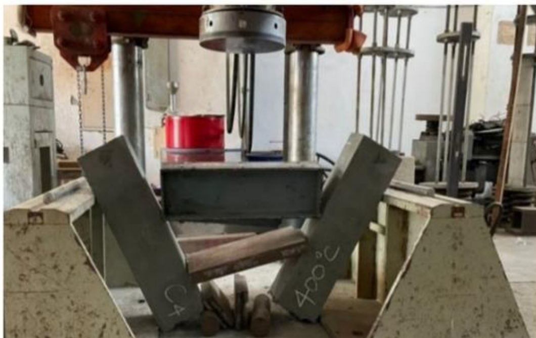
Figure 5: The fracture situation of the experimental group after being subjected to 400 °C.
