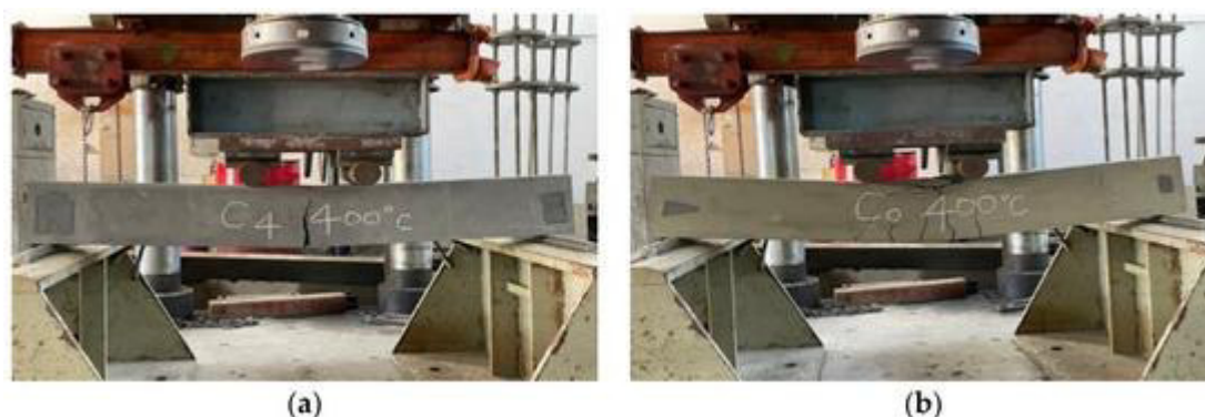
Figure 4: The tensile failure in the flexural test of beams after being subjected to 400 °C: (a) the experimental group and (b) the control group.
