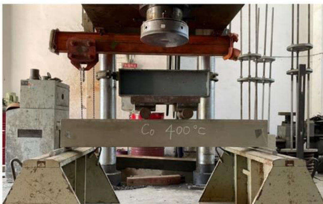
Figure 2: The general flexural test setup for the beam specimens.
