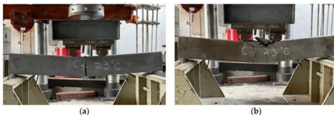
Figure 3: The tensile failure in the flexural test of beam at room temperature: (a) the experimental group and (b) the control group.
