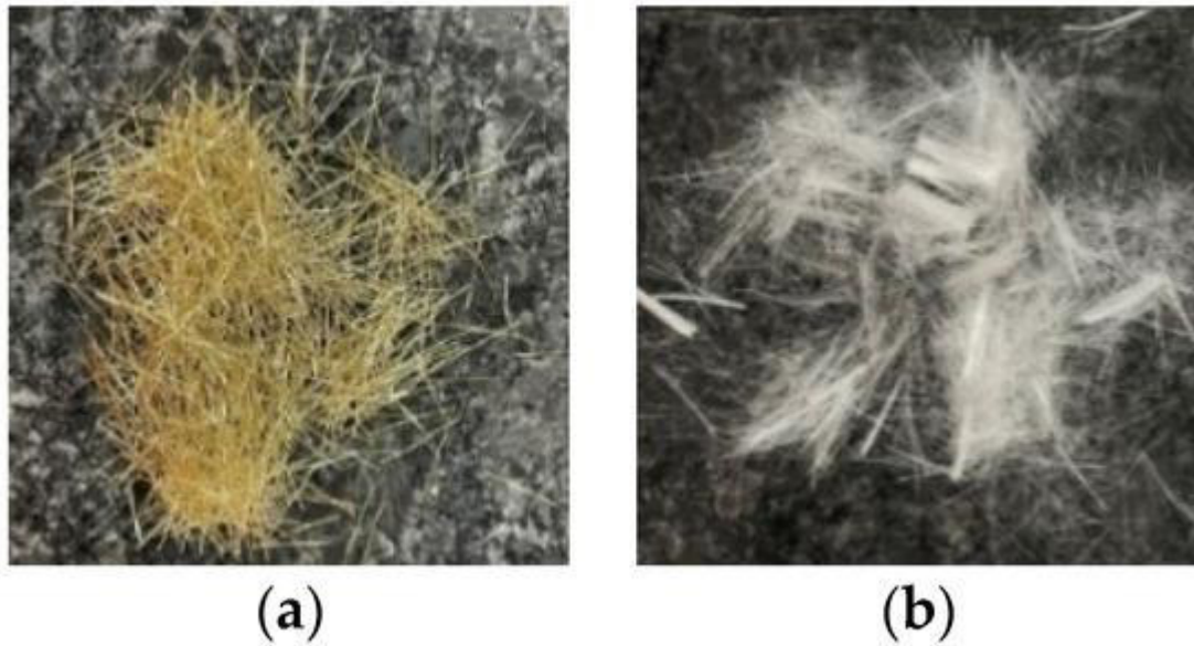
Figure 1: The appearance of the fibers: (a) steel fibers and (b) polypropylene fibers.
